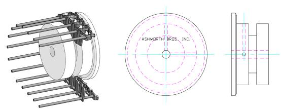
Support rollers are still recommended between flanged idlers. To calculate the maximum diameter of the support rolls, use the formula in the previous section substituting the sum of the hub diameter of the chosen flanged idler + .590 inches (one link height) for the PD (pitch diameter).
