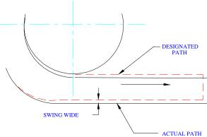
Ashworth recommends a minimum swing wide clearance of 1 inch per foot of width [75 mm per meter of width] be built into all conveyors where the belt enters or exits a turn.
