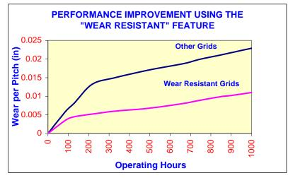
Provides a flatter mesh surface with a high resilience to impact.
